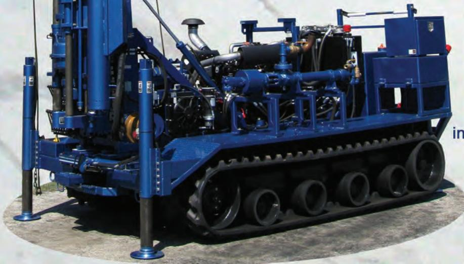
The D-120 is a large, heavy-duty, high power, multi-purpose drill rig. This drill has earned a reputation as a powerhouse in the geotechnical, exploration and environmental drilling industries. The D-120 is powerful enough to handle large diameter hollow stem augers, yet versatile enough to drill efficiently on small auger, rotary and core jobs. If you need more power, more capacity and more productivity, the D-120 is the drill for you!
