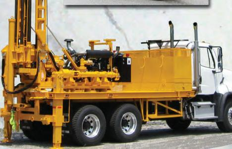
The D-90 is a large, heavy-duty multi-purpose drill rig used for soil and rock sampling for both geotechnical, exploration and environmental investigations using augers, mud rotary or core drilling tools. With various mounting and drill options avaliable, the D-90 is one versatile drill rig!
